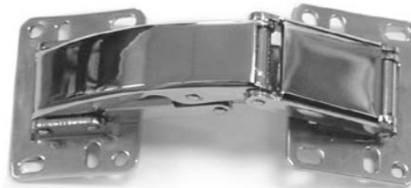
#42.7753; 125 degree 316 stainless steel easy on hinge
